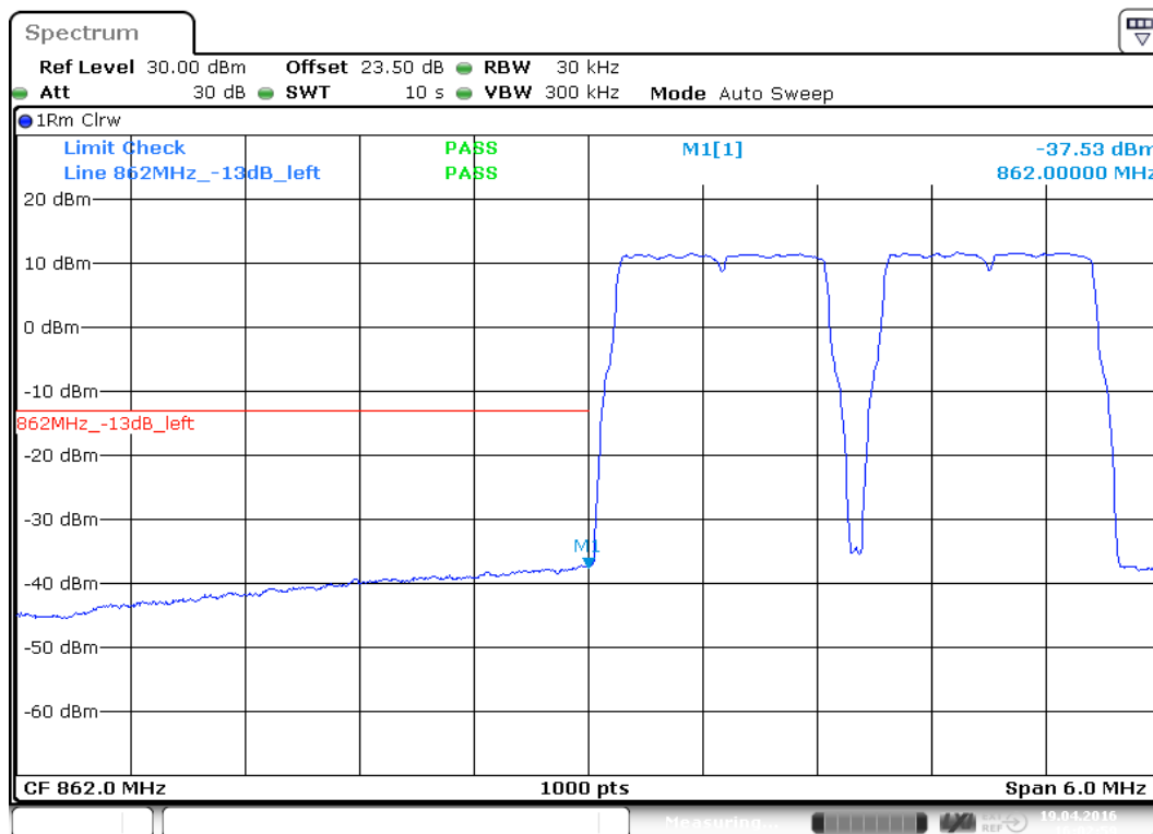
plot 8.3.1.5-#1 Intermodulation: §90.219, §2.1051; Test results; Downlink; LTE Lower Band Edge
