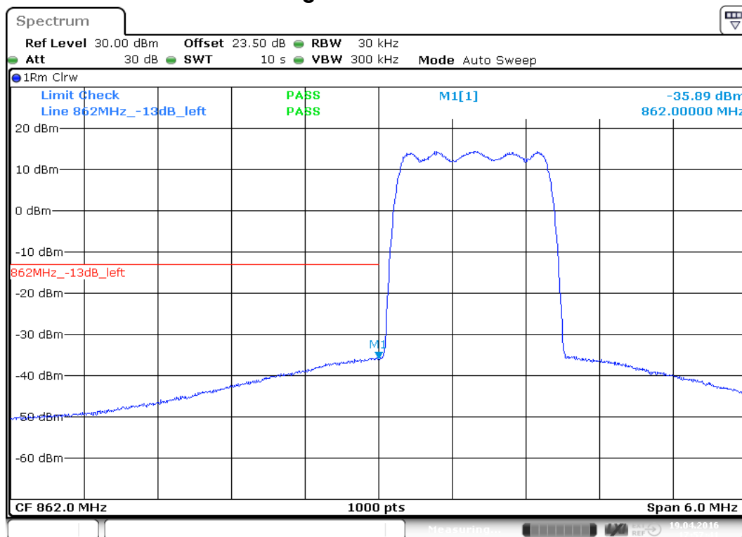
plot 9.3.1.3-#1 Emission Mask: §90.691, §2.1051; Test results; Downlink; CDMA < 1MHz to band edge Lower Band Edge
