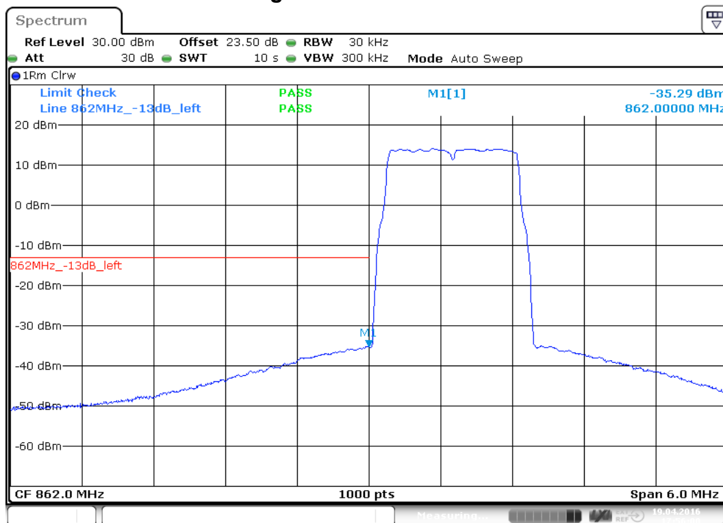
plot 9.3.1.5-#1 Emission Mask: §90.691, §2.1051; Test results; Downlink; LTE < 1MHz to band edge Lower Band Edge
