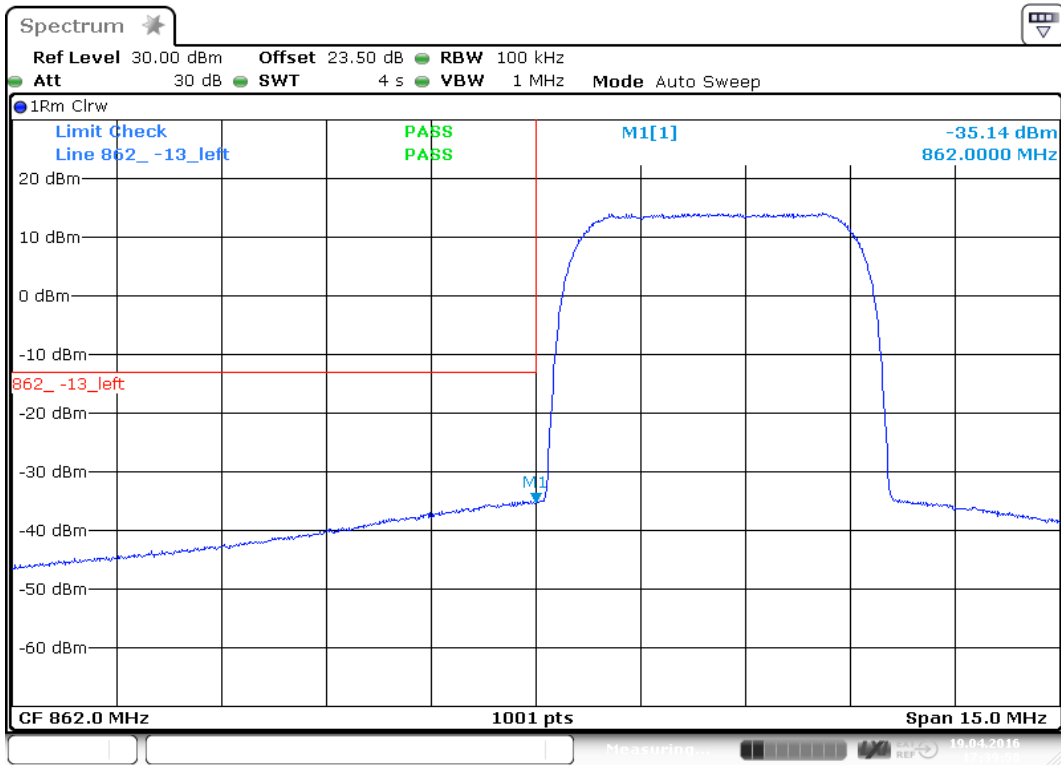
plot 9.3.1.4-#1 Emission Mask: §90.691, §2.1051; Test results; Downlink; WCDMA < 1MHz to band edge Lower Band Edge
