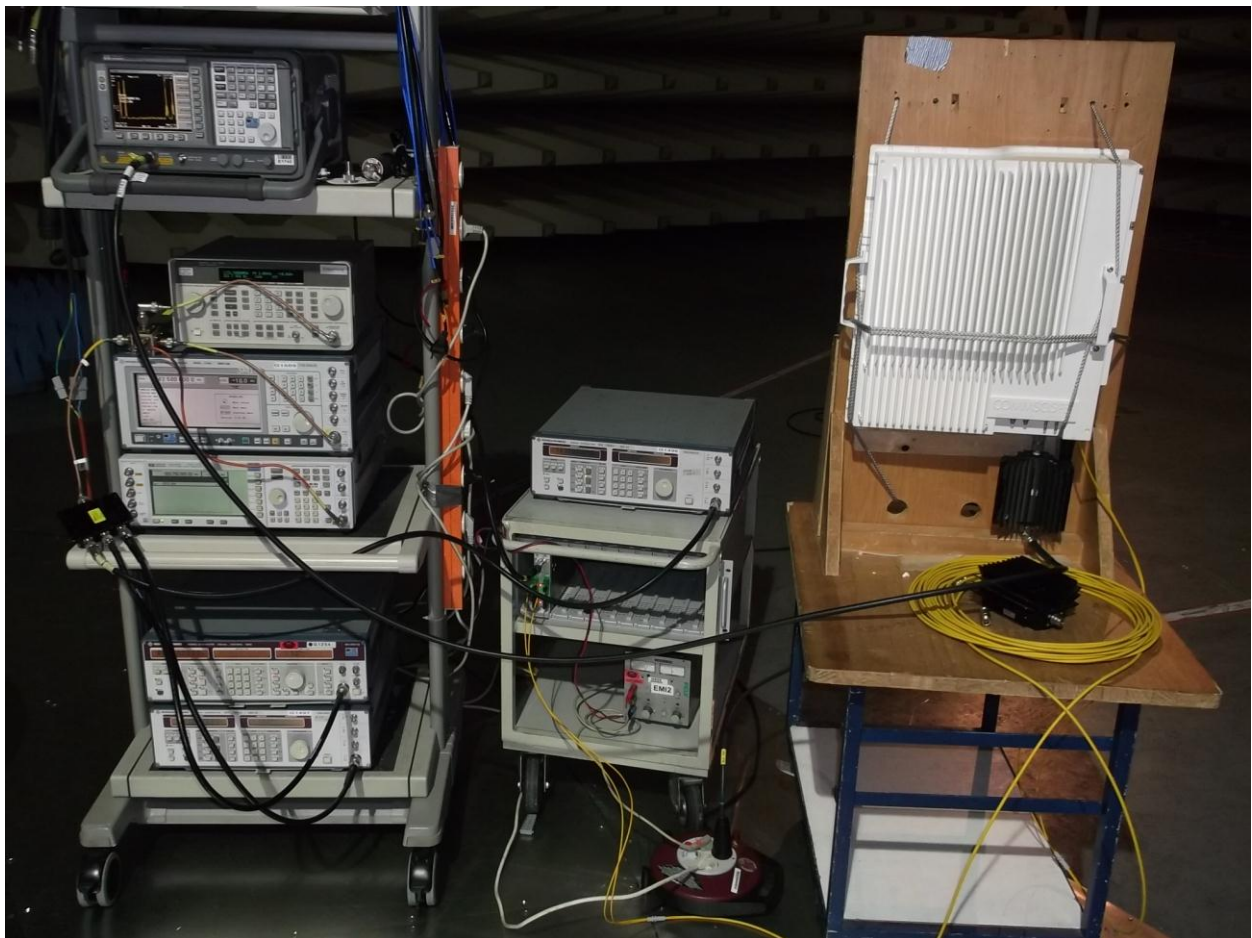
picture 8.2: Test setup: Field Strength Emission in the SAC
