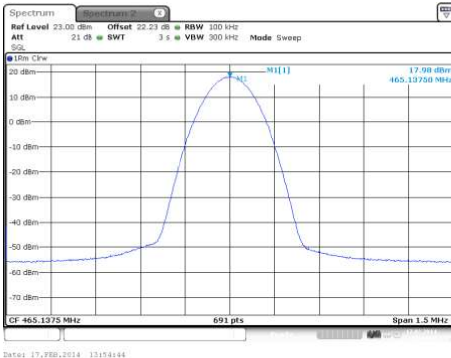
plot 5.3.1.3-#1 RF Power Out: §90.219, §2.1046; Test Results; Downlink; Band # 3; APCO Phase2 H-DQPSK
