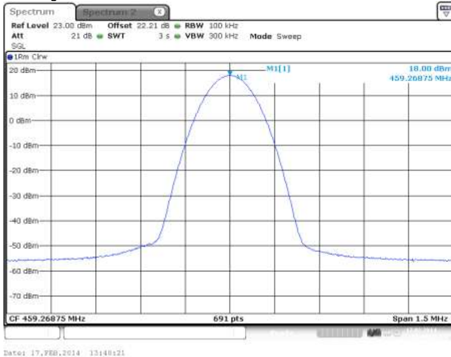
plot 5.3.1.2-#1 RF Power Out: §90.219, §2.1046; Test Results; Downlink; Band # 2; Analog
