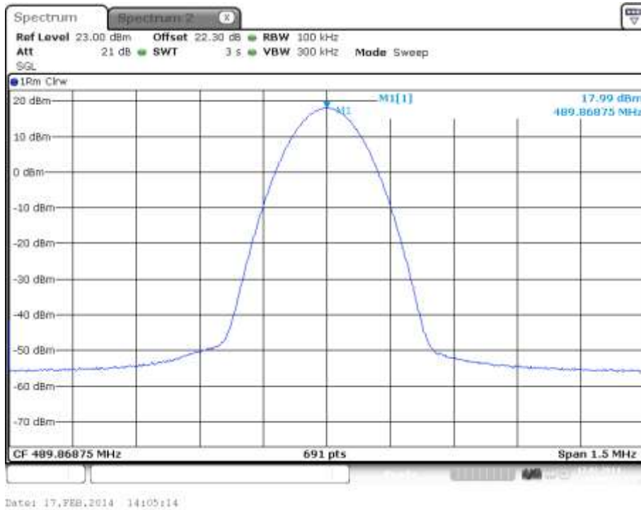
plot 5.3.1.4-#1 RF Power Out: §90.219, §2.1046; Test Results; Downlink; Band # 4; APCO Phase1 C4FM
