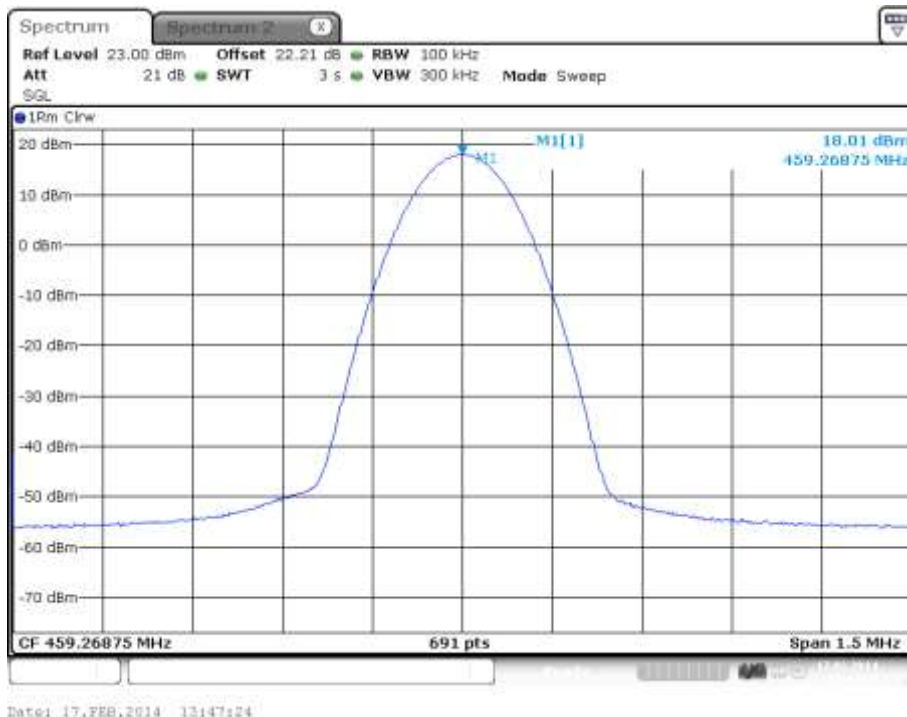
plot 5.3.1.2-#1 RF Power Out: §90.219, §2.1046; Test Results; Downlink; Band # 2; APCO Phase1 C4FM
