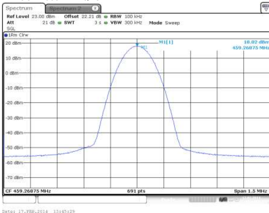
plot 5.3.1.2-#1 RF Power Out: §90.219, §2.1046; Test Results; Downlink; Band # 2; APCO Phase2 H-DQPSK
