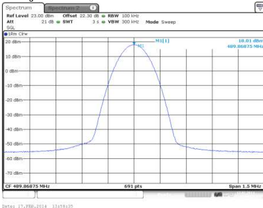
plot 5.3.1.4-#1 RF Power Out: §90.219, §2.1046; Test Results; Downlink; Band # 4; Analog
