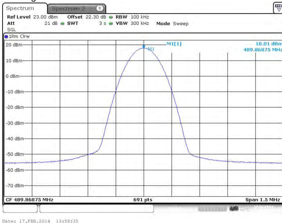
plot 5.3.1.4-#1 RF Power Out: §90.635, §2.1046; Test Results; Downlink; Band # 4; Analog
