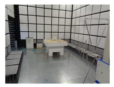
Figure 9.1-3: Radiated emissions set-up for frequencies below 1 GHz
