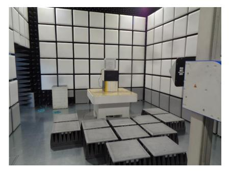
Figure 9.1-4: Radiated emissions set-up for frequencies above 1 GHz
