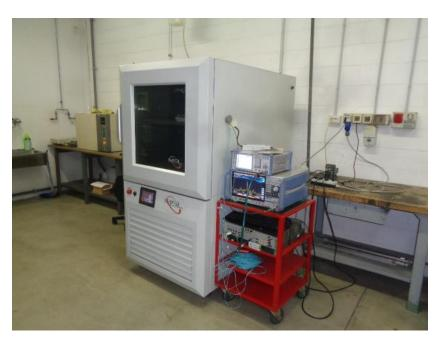
Figure 9.1-2: Antenna port testing set-up in climatic chamber
