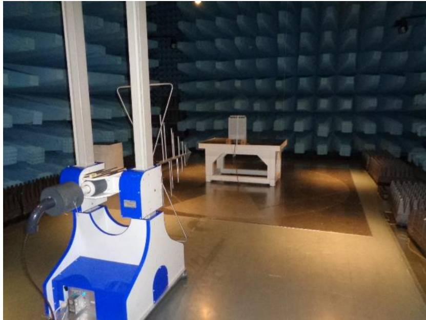
Figure 9.1-3: Radiated emissions set-up for frequencies below 1 GHz
