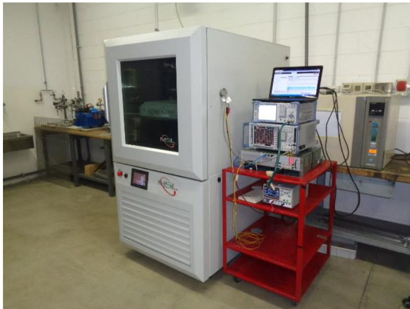
Figure 9.1-2: Antenna port testing set-up in climatic chamber
