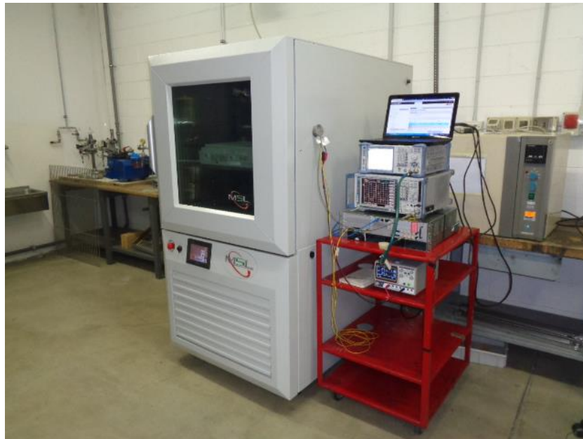
Figure 9.1-2: Antenna port testing set-up in climatic chamber
