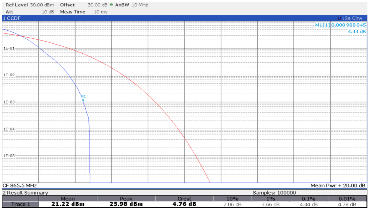
Figure 8.4-11: PAPR at antenna port 2 with input signal at AGC threshold
