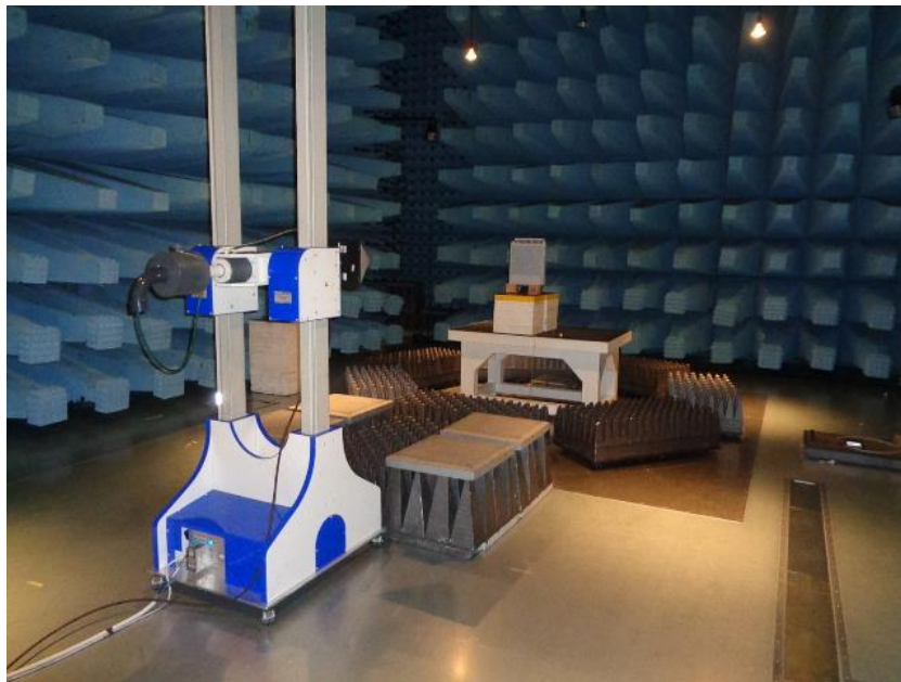
Figure 9.1-4: Radiated emissions set-up for frequencies above 1 GHz
