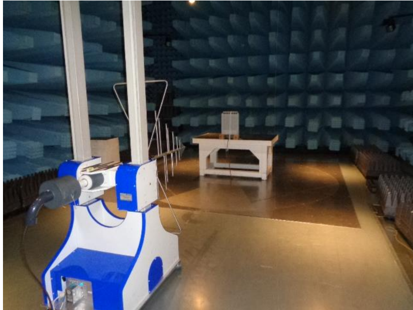
Figure 9.1-3: Radiated emissions set-up for frequencies below 1 GHz
