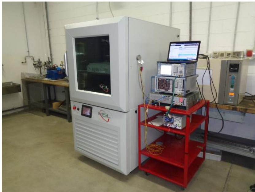
Figure 9.1-2: Antenna port testing set-up in climatic chamber
