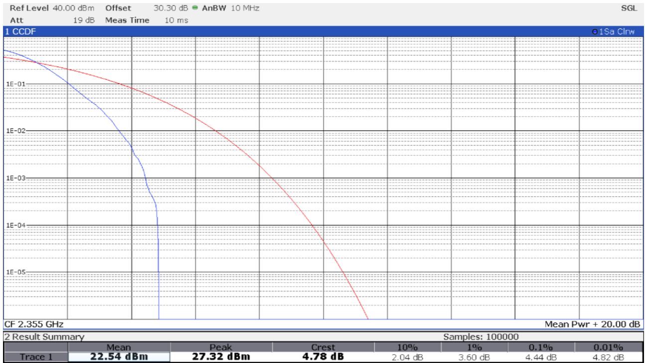
Figure 8.4-12: PAPR at antenna port 2 with input signal at AGC threshold +3 dB
