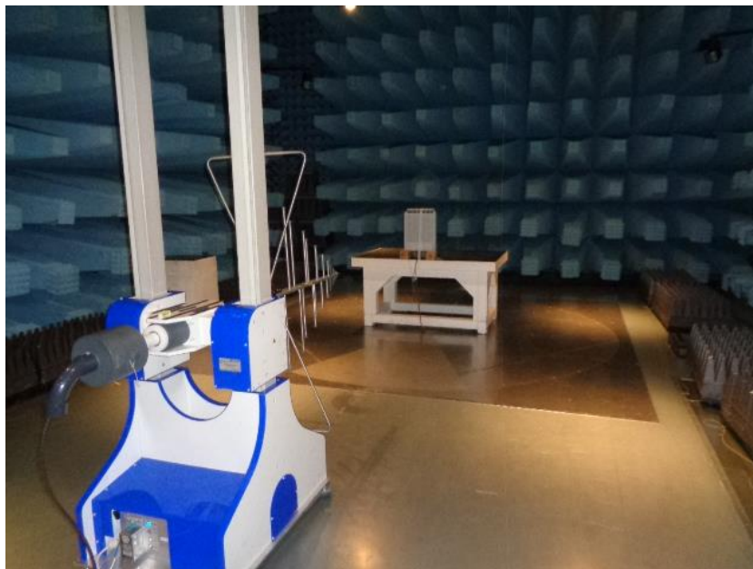
Figure 9.1-3: Radiated emissions set-up for frequencies below 1 GHz
