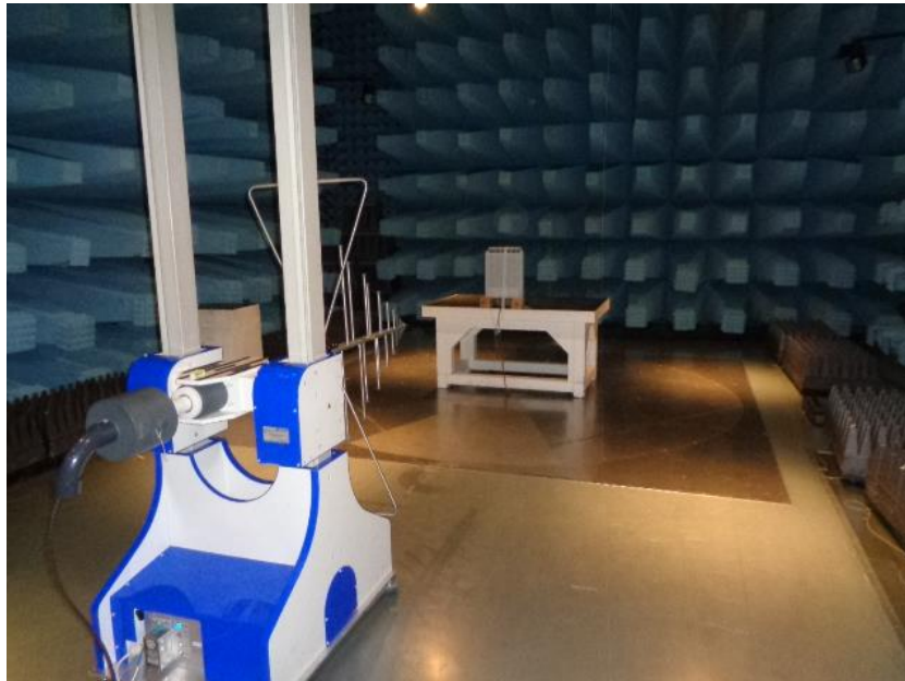
Figure 9.1-3: Radiated emissions set-up for frequencies below 1 GHz
