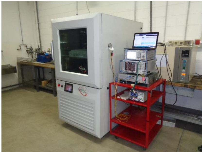
Figure 9.1-2: Antenna port testing set-up in climatic chamber
