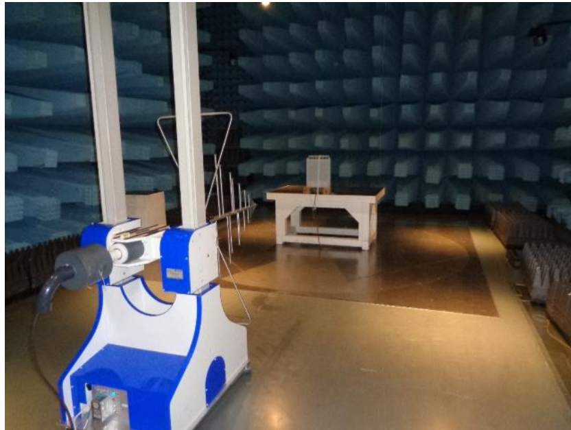
Figure 9.1-3: Radiated emissions set-up for frequencies below 1 GHz
