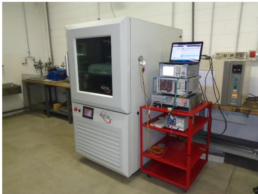
Figure 9.1-2: Antenna port testing set-up in climatic chamber
