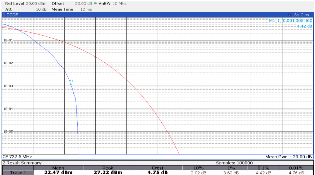
Figure 8.4-9: PAPR at antenna port 1 with input signal at AGC threshold
