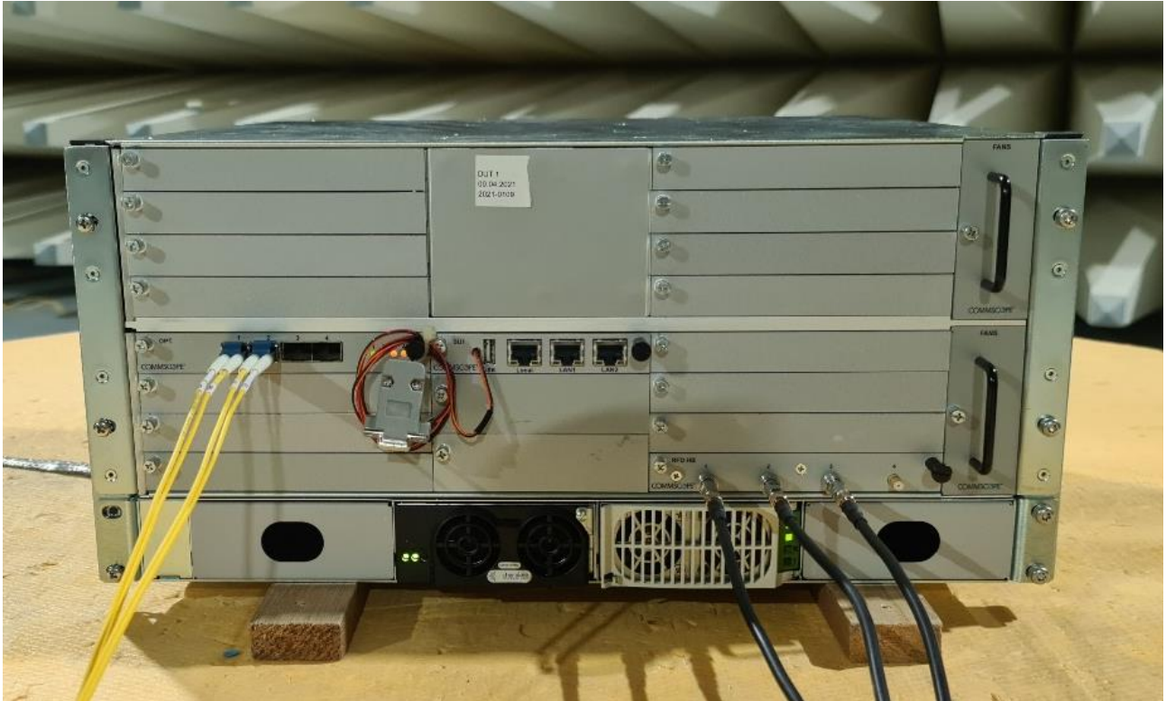
Photograph 9: Photograph of ION-E WCS-4 Subrack frontside
