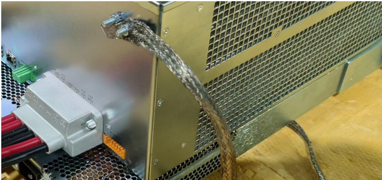
Photograph 2: Photograph of DUT's grounding
