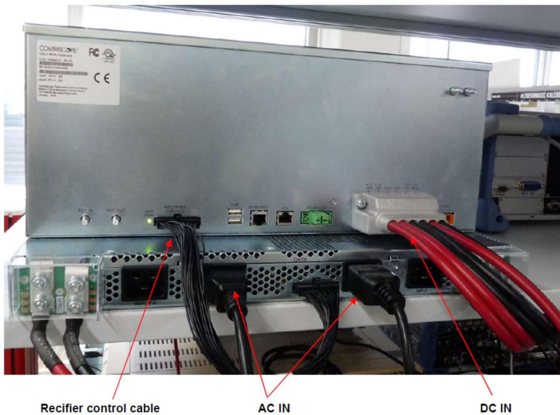
Photograph 10: Photograph of ION-E WCS-4 Subrack backside
