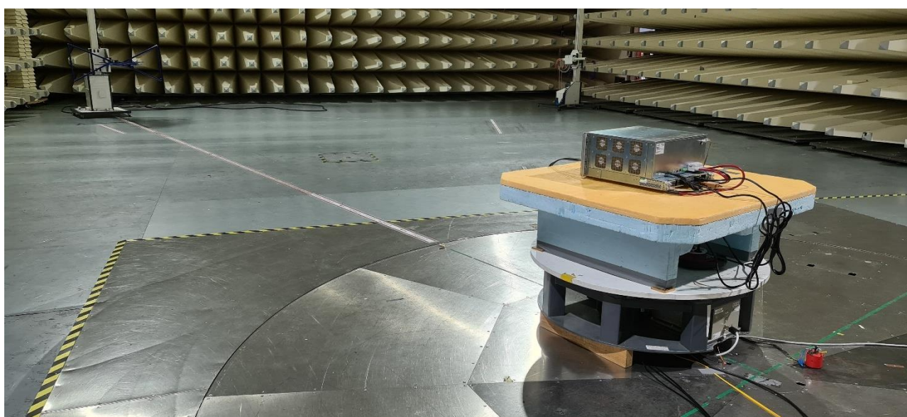
Photograph 4: Setup of radiated emissions measurement in the frequency range 30 – 1000 MHz
