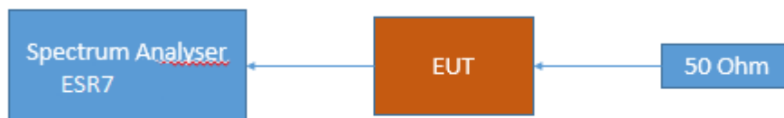
FCC Part 22/24/27/90 Industrial signal booster – Test Setup; Noise
