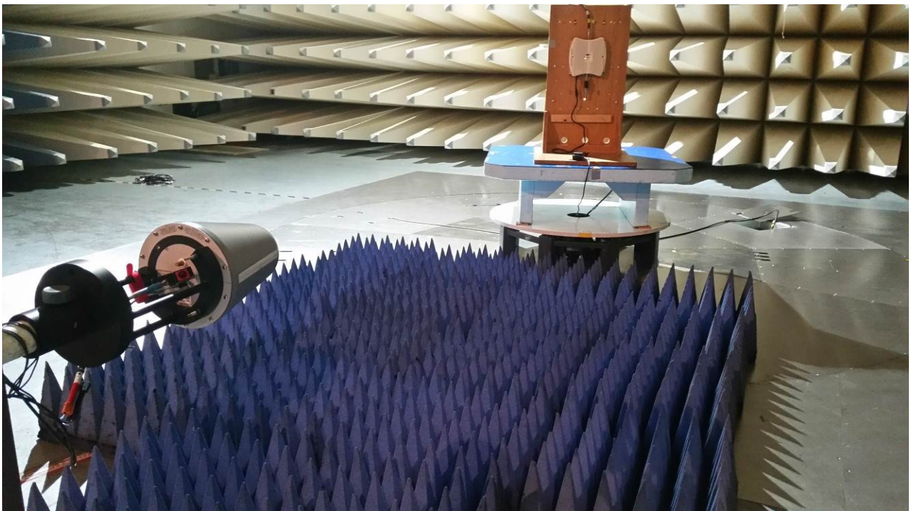
picture 8.4: Test setup: Field Strength Emission 1 – 18 GHz @3m in the SAC
