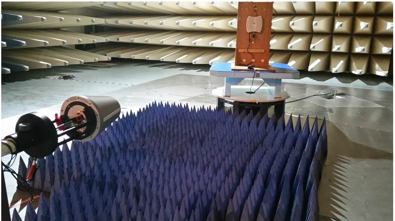
Test setup: Field Strength Emission 1 – 18 GHz @3m in the SAC
