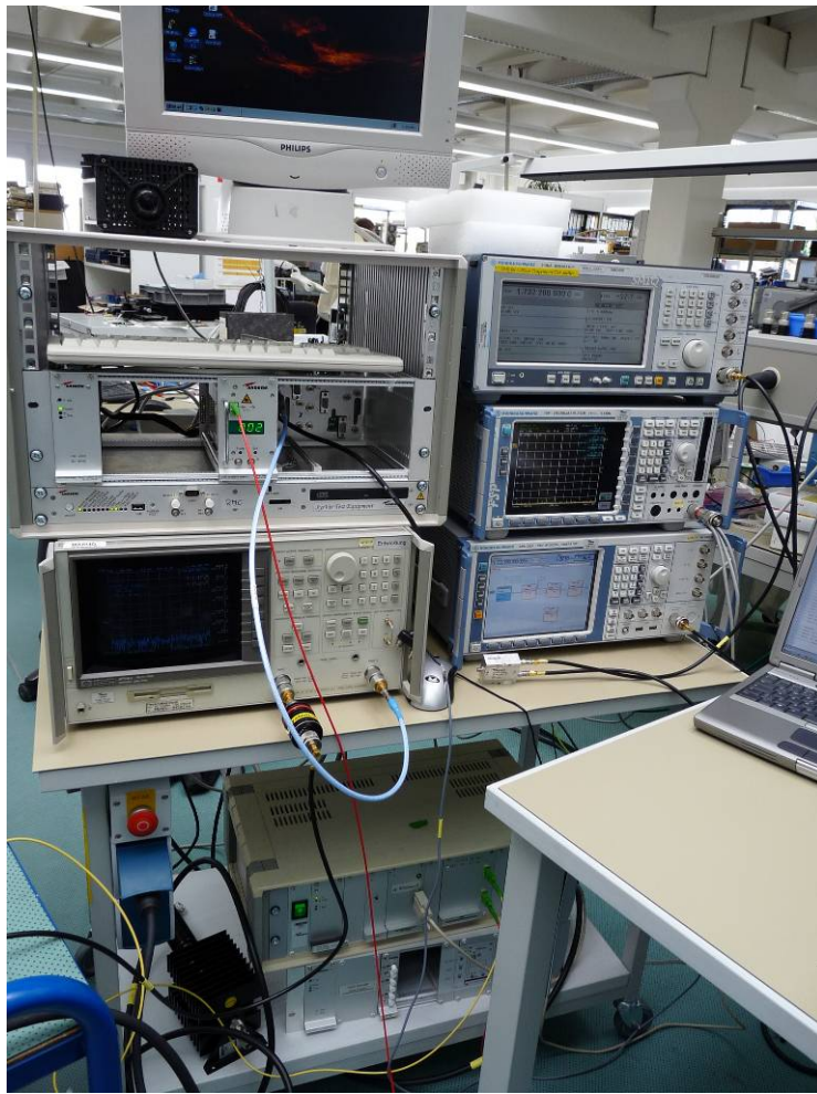
Figure 2. Measurement Equipment and Remote Unit
