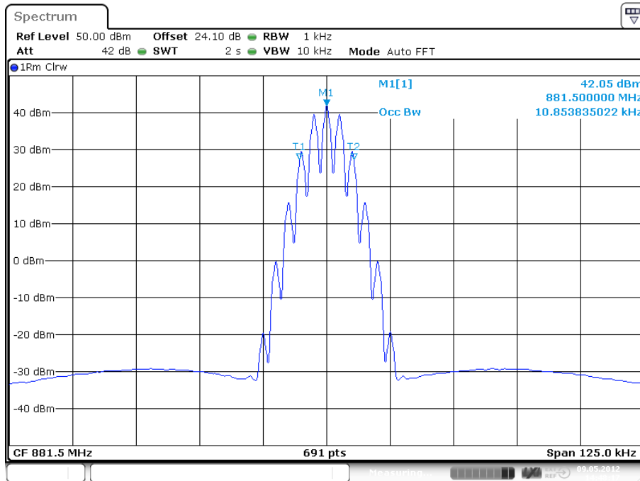
plot 6.3.1.1-#1 Occupied Bandwidth: $2.1049; RSS-GEN; Test results; Downlink; Analog Output
