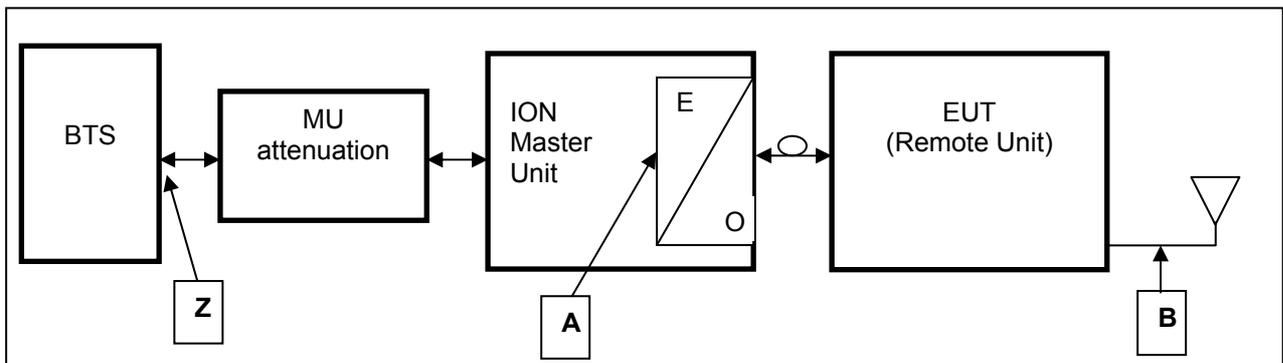
figure 2.1.5-#1 Block diagram of measurement reference points
