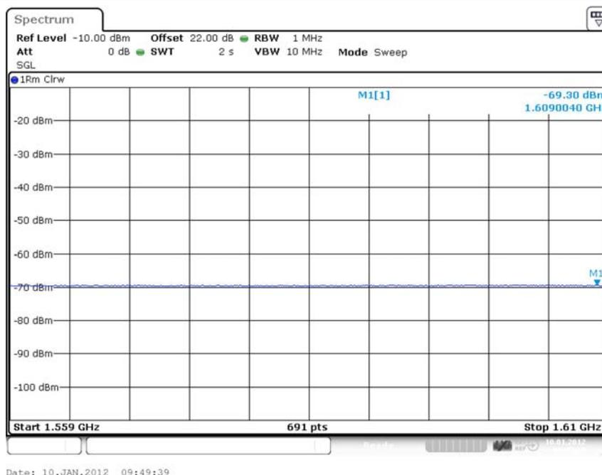
plot 8.5.7.3 Spurious Emissions at Antenna Terminals; Measurement in the band of 1559 MHz – 1610 MHz; Measurement in the band of 1559 – 1610 MHz
