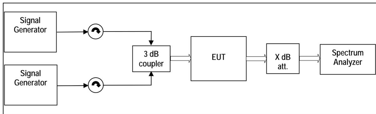
figure 8-#1 Test setup: Radiated Spurious Emissions at the ECL (TEMPTON): §27.53, §2.1053, RSS-Gen, RSS-131
