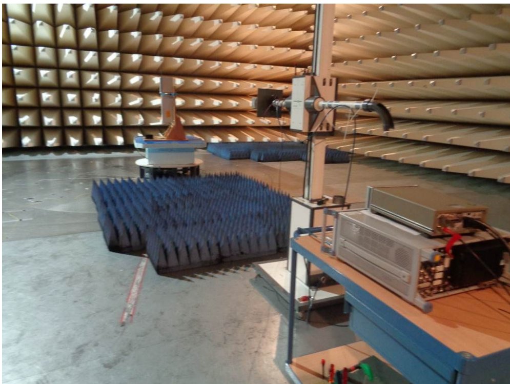
Test setup: Field Strength Emission 18 – 26.5 GHz @3m in the SAC
