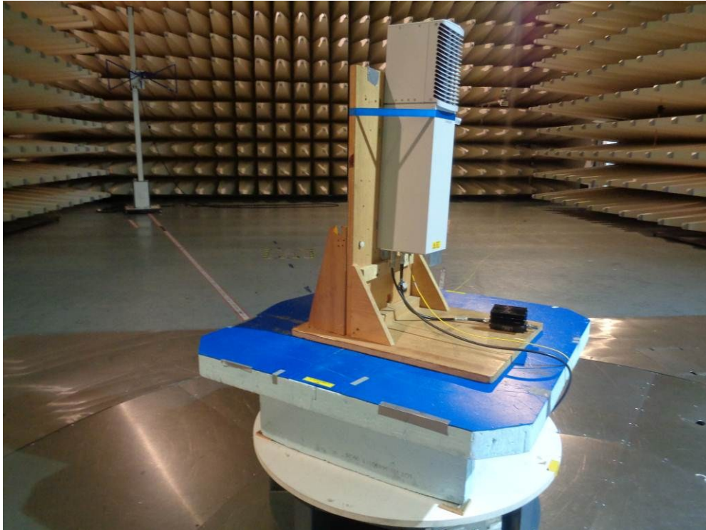
Test setup: Field Strength Emission 30 M – 1 GHz @10m in the SAC
