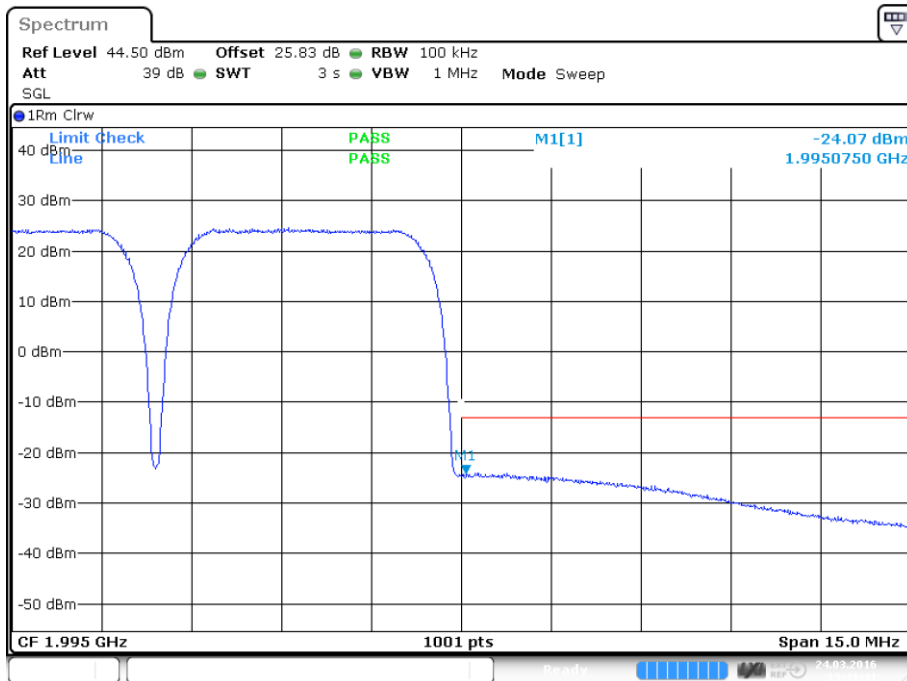
plot 8.3.1.4-#1 Intermodulation: §24.238, §2.1051; Test results; Downlink; WCDMA Lower Band Edge
