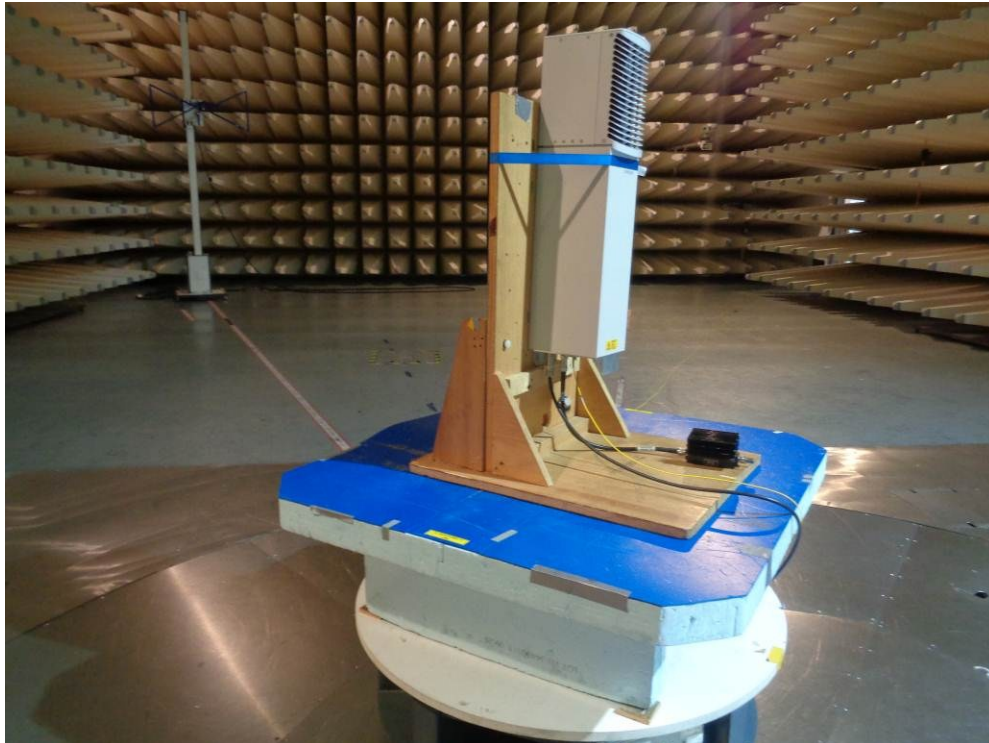
picture 8.2: Test setup: Field Strength Emission 30 M – 1 GHz @10m in the SAC
