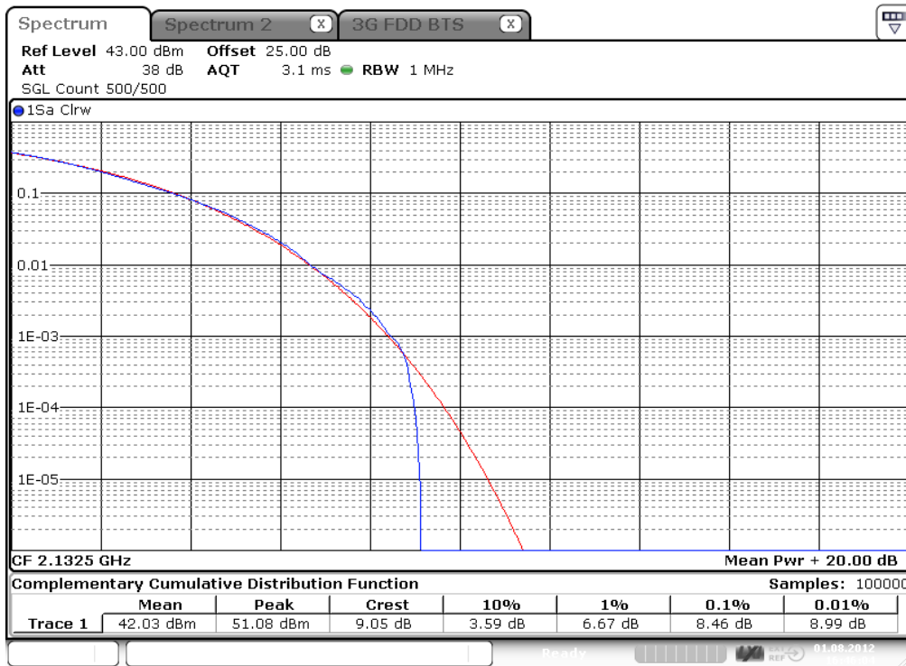
plot 8.3.1.3-#1 Transmitter Output Power: IC RSS-139, RSS-GEN; Test results; Downlink; LTE Middle Peak - to - average
