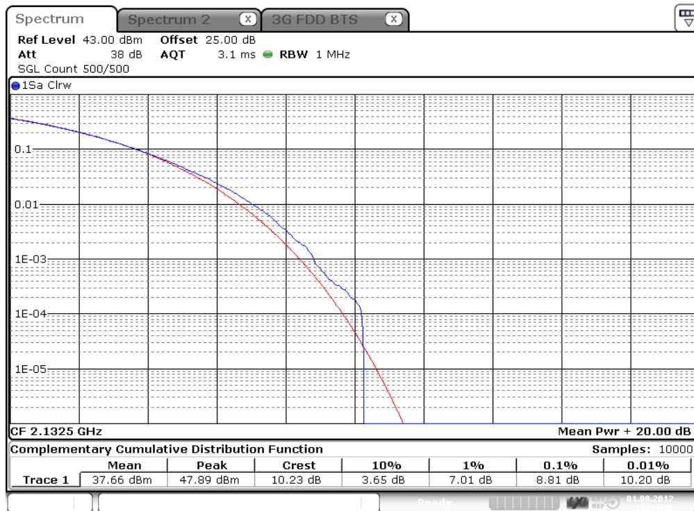
plot 8.3.1.2-#1 Transmitter Output Power: IC RSS-139, RSS-GEN; Test results; Downlink; WCDMA Middle Peak - to - average
