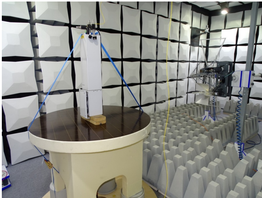
Photo 3: Test setup for radiated emissions measurements in fully-anechoic chamber (1 GHz to 22 GHz), rear side view, EUT vertical
