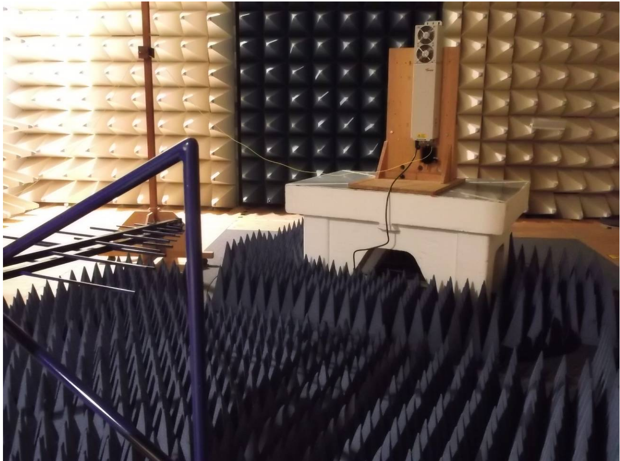
picture 8.2: Test setup: Field Strength Emission <1 GHz @3m in the FAC
