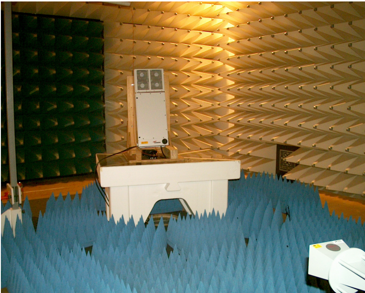
picture 8.3: Test setup: Field Strength Emission >20 GHz @3m in the FAC with Absorber material
