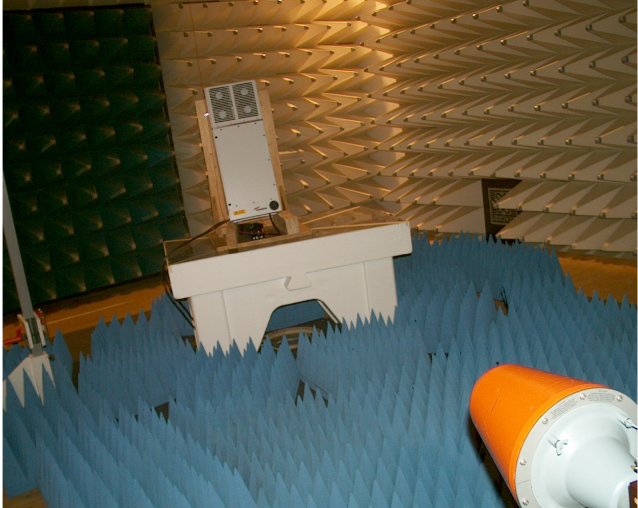
picture 8.1: Test setup: Field Strength Emission 1GHz to 20GHz @3m in the FAC
