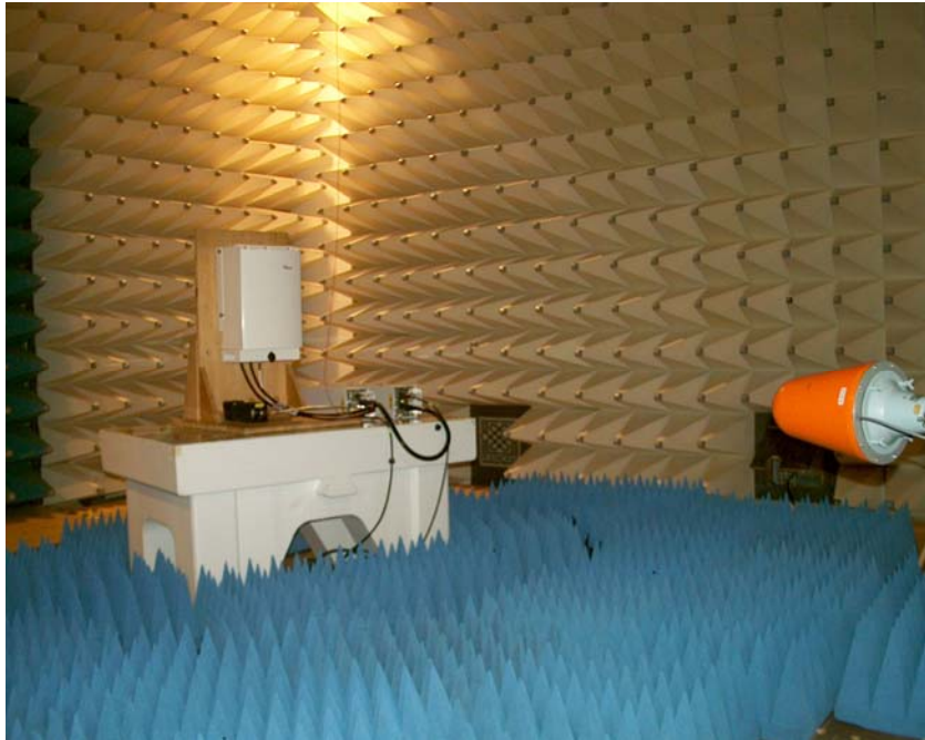
picture 7.1: Test setup: Field Strength Emission >1 GHz @3m in the FAC
