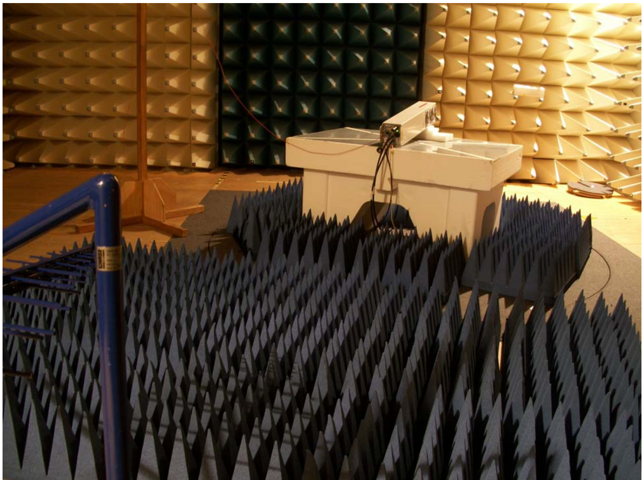
picture 8.3: Test setup: Field Strength Emission <1 GHz @3m in the FAC
