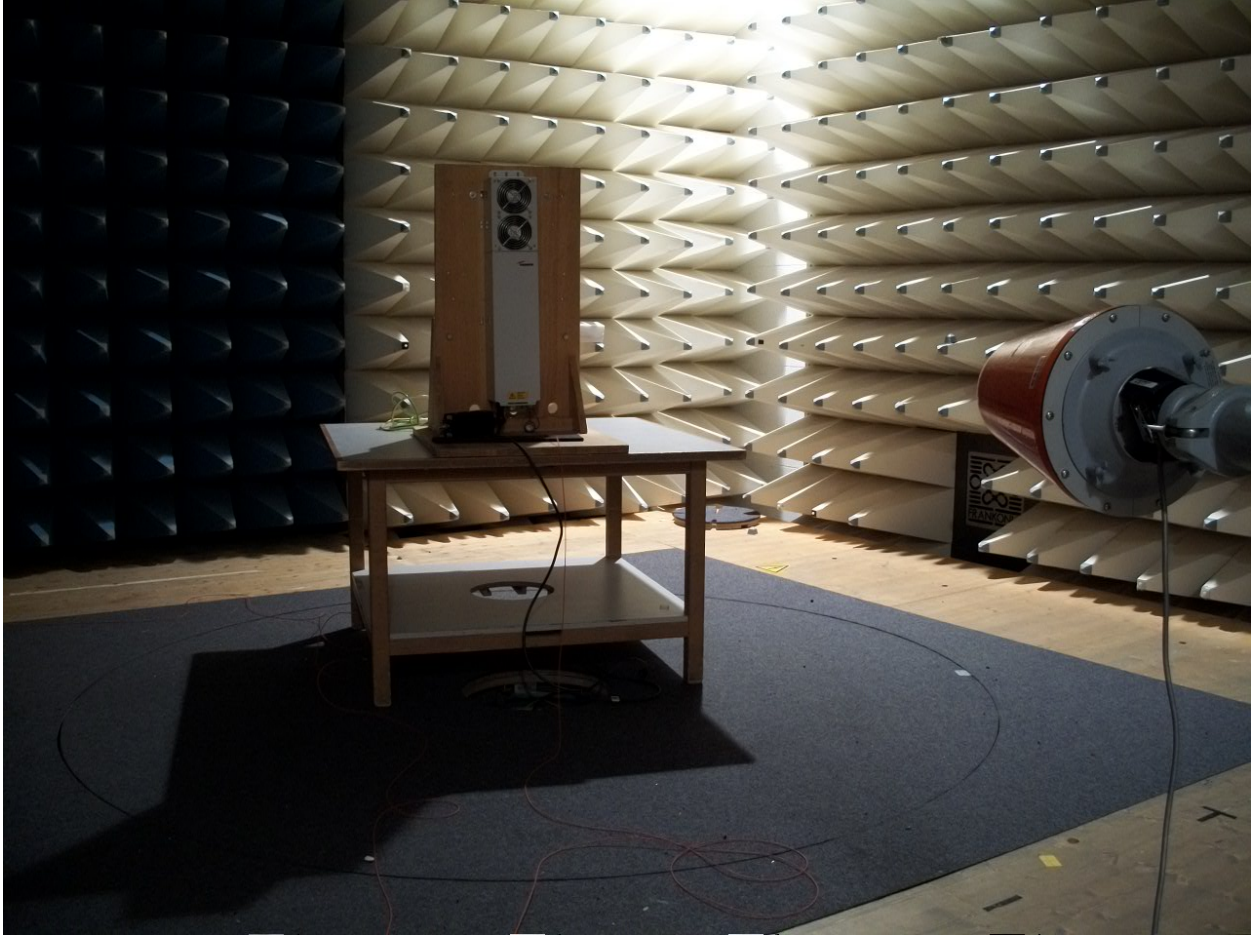
picture 8.1: Test setup: Field Strength Emission 1GHz to 20GHz @3m in the FAC
