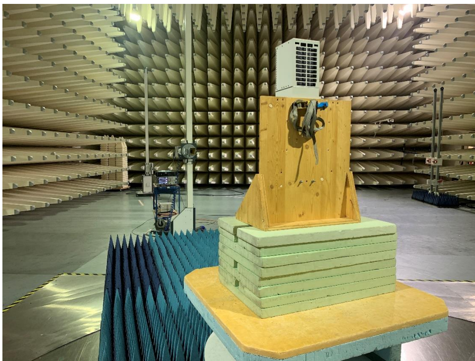
Photograph 7: Setup of radiated emissions measurement in the frequency range from 18 GHz to 26 GHz.
