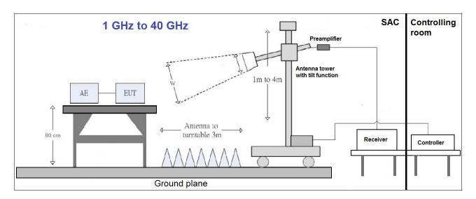
The following modifications apply to the measurement procedure for the frequency range above 1 GHz:
