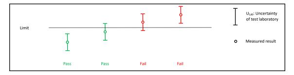
There is a risk of a "False Accept" as well as a "False Reject" when the measured value plus the measurement uncertainty U<sub>Lab</sub> is above respectively below the specification limit.
