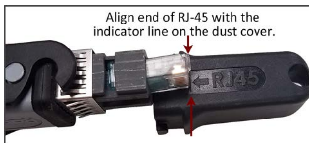
Figure 11. RJ-45 Dust Cover Alignment
