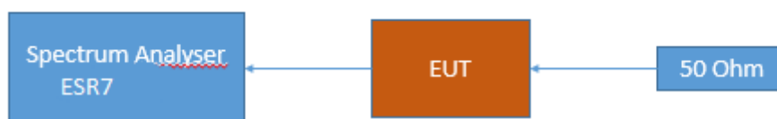
FCC Part 22/24/27/90 Industrial signal booster – Test Setup; Noise
