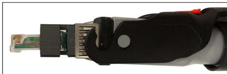
Figure 14. GigaSPEED X10D RJ-45 Correctly Installed in OCTIS Connector
