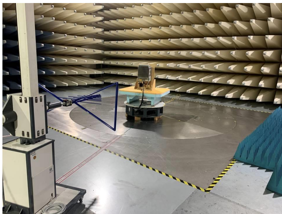
Photograph 2: Setup of radiated emissions measurement in the frequency range 30 – 1000 MHz
