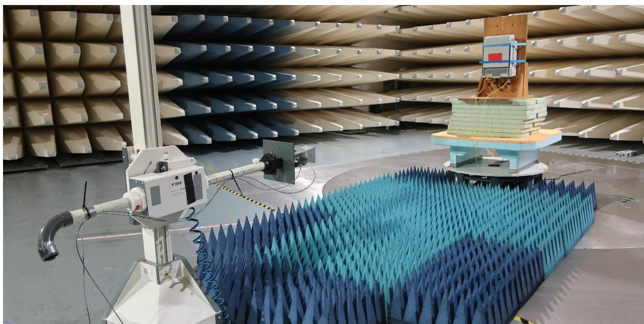
Photograph 7: Setup of radiated emissions measurement in the frequency range from 18 GHz to 26 GHz.
