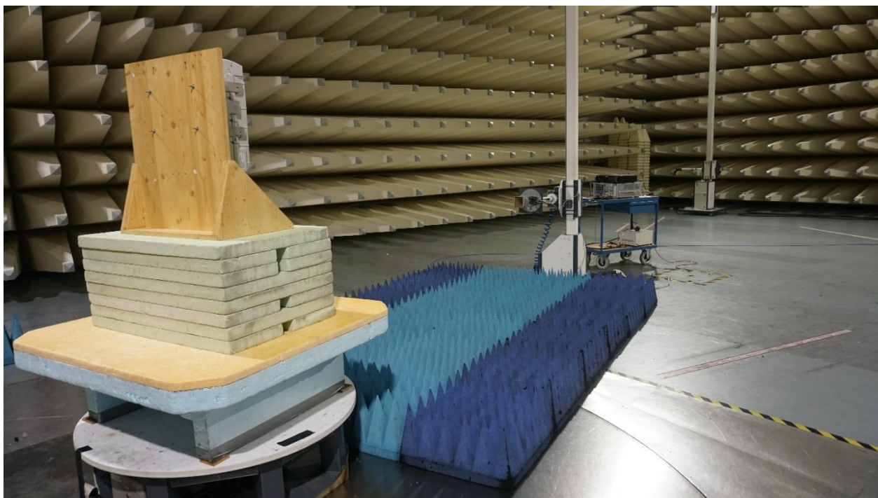
Photograph 7: Setup of radiated emissions measurement in the frequency range from 18 GHz to 27 GHz.
