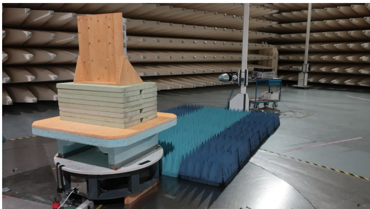
Photograph 5: Setup of radiated emissions measurement in the frequency range from 1 GHz to 18 GHz.
