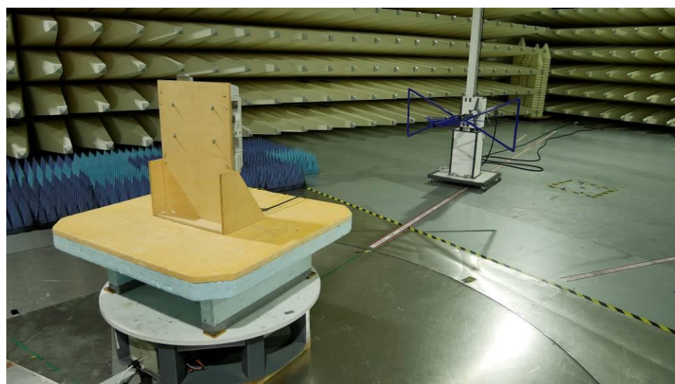
Photograph 3: Setup of radiated emissions measurement in the frequency range 30 – 1000 MHz
