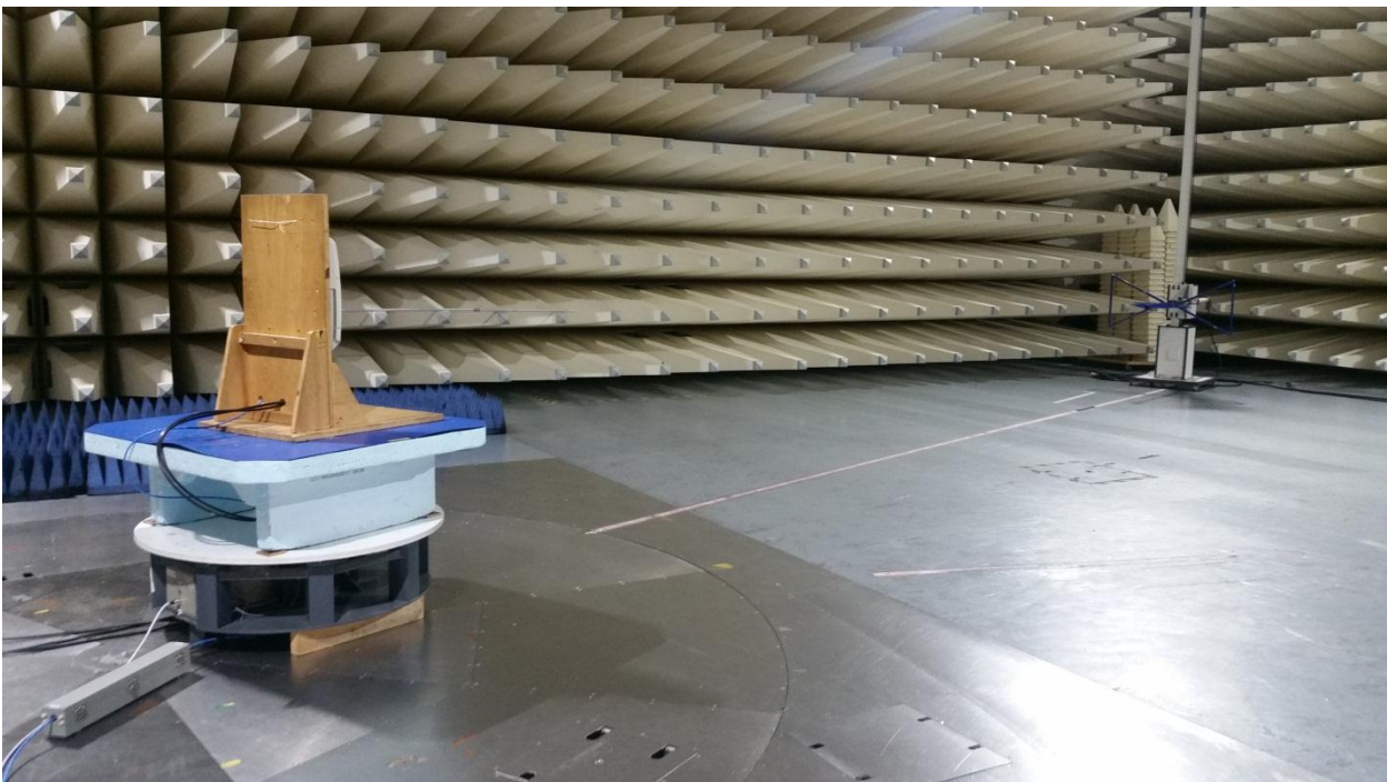
picture 8.2: Test setup: Field Strength Emission <1 GHz @10m in the SAC
