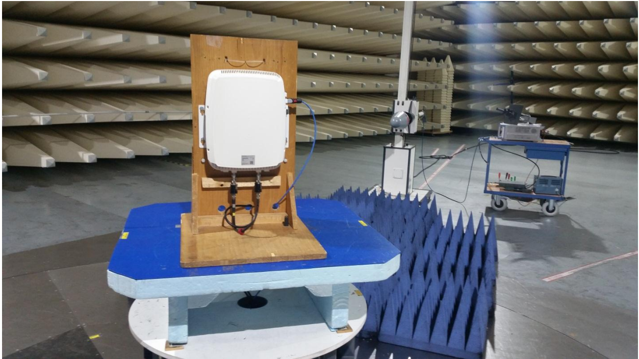
picture 8.3: Test setup: Field Strength Emission 1 - 18 GHz @3m in the SAC
