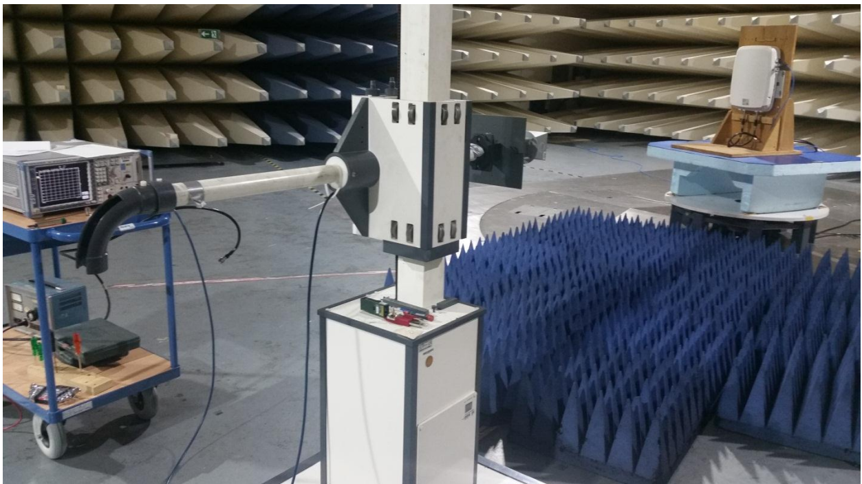
picture 8.4: Test setup: Field Strength Emission 18 – 26,5 GHz @3m in the SAC
