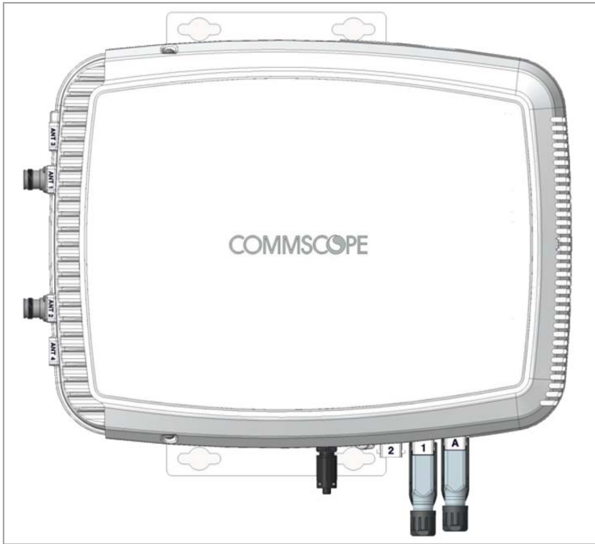
Figure 7-5. Mounting Orientation for a CAP L with the Optional Fan Kit (Flat Mounting Bracket Shown)
