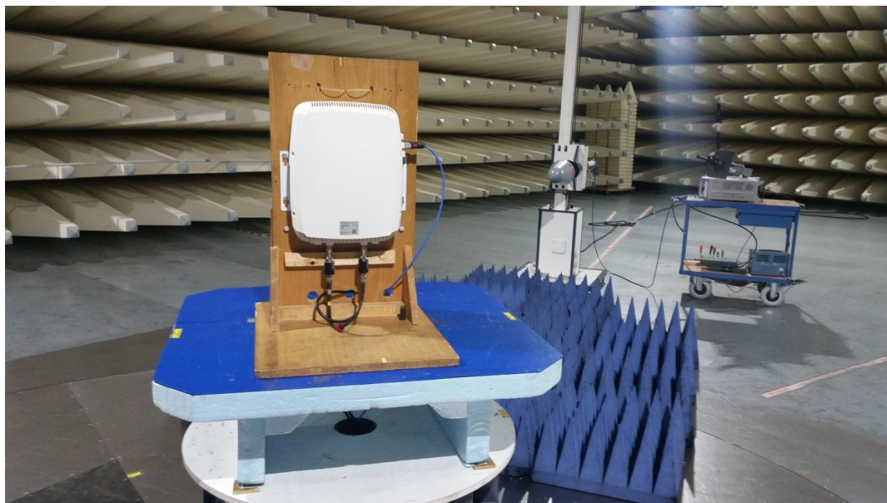
picture 8.3: Test setup: Field Strength Emission 1 - 18 GHz @3m in the SAC
