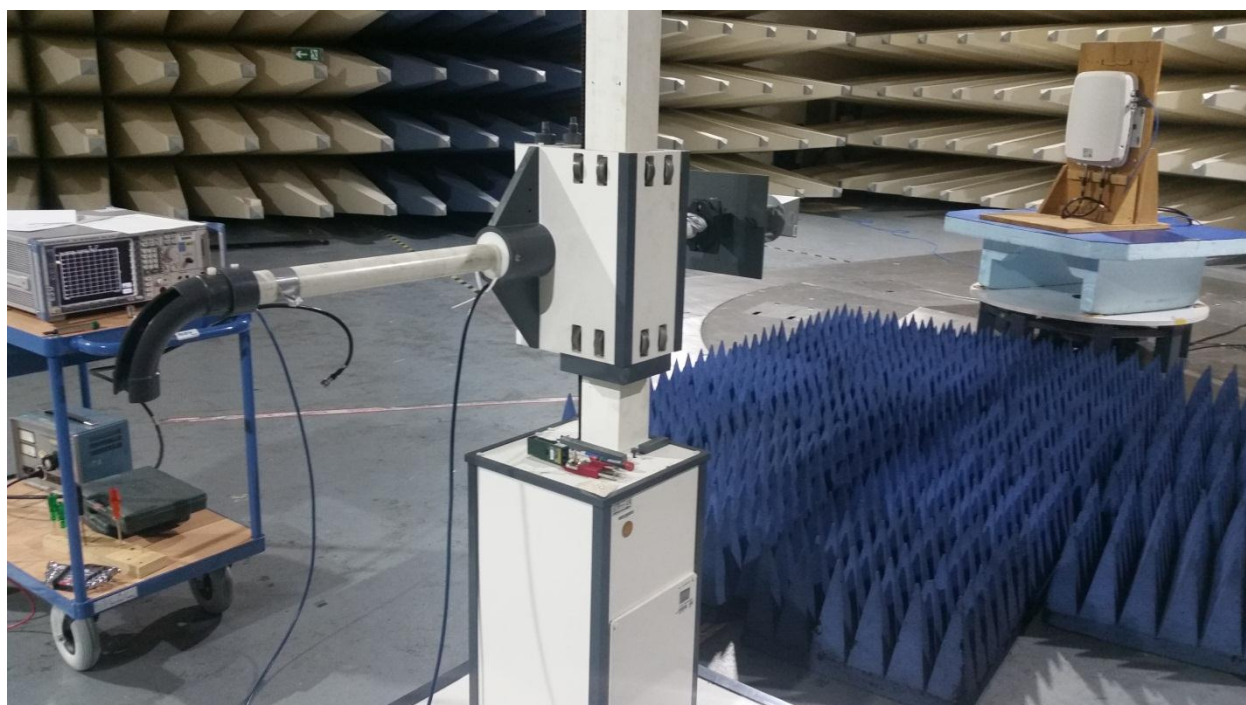
picture 8.4: Test setup: Field Strength Emission 18 - 26,5 GHz @3m in the SAC
