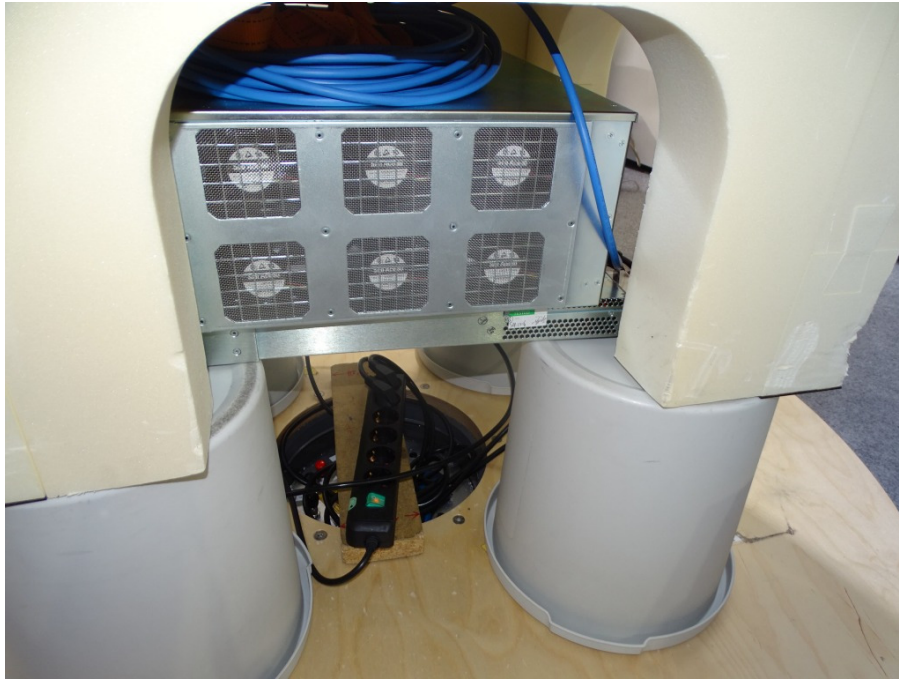
Photo 5: Test setup for radiated emissions measurements in fully-anechoic chamber (1 GHz to 10/20 GHz), front side view (auxiliary equipment below table)
