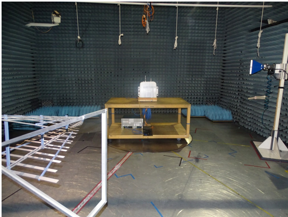
Photo 2: Test setup for radiated emissions measurements in semi-anechoic chamber (30 MHz to 1 GHz), front side view (with auxiliary equipment below table)
