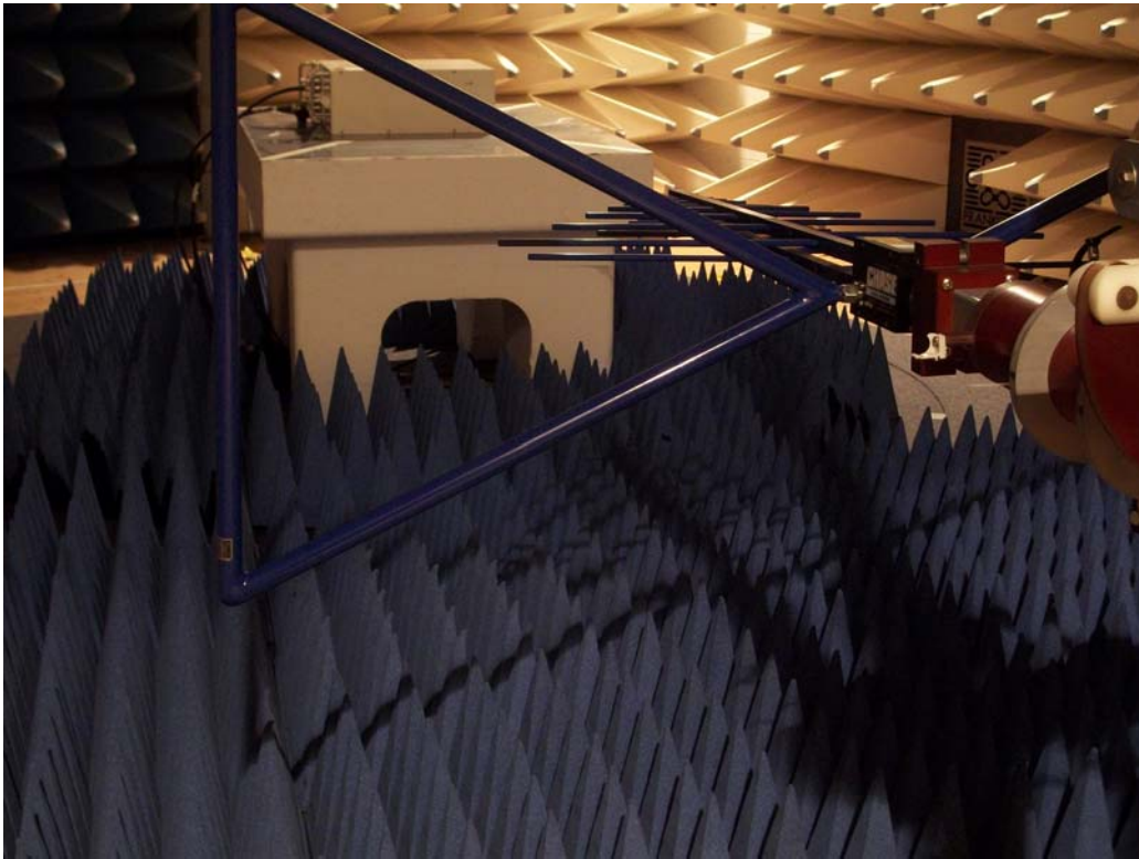
picture 8.5: Test setup: Field Strength Emission <1 GHz @3m in the FAC
