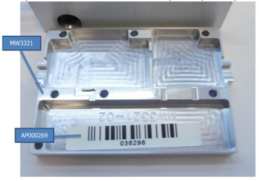
5) Record internal RF card PCBA serial number, then route to enclosure.
