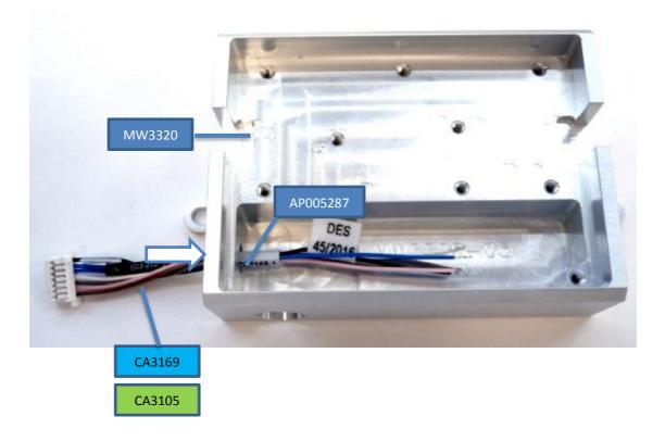
For the Mesh products insert cable assembly (CA3105) loom through PV5 Grommet (AP005287) and the hole.
