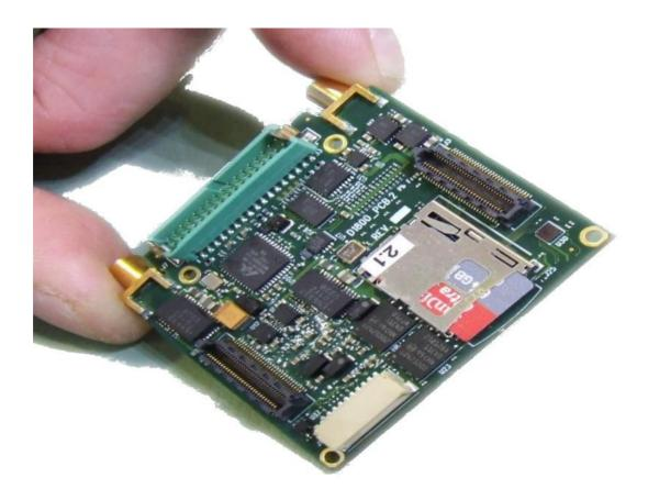
10) Connect the **SA4130** to the **D18xx** or **D1896** PCBA. Carefully align to the pillars and pressure evenly.
