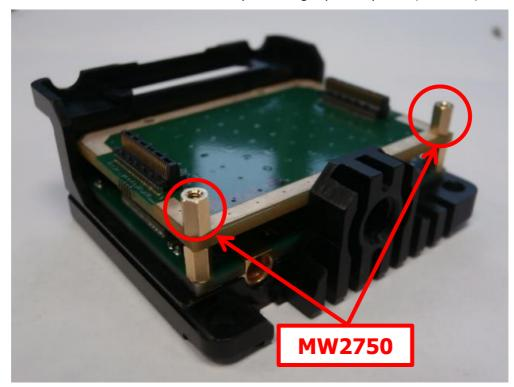
8) UHF ONLY: Now fit to the RF card. Secure in place using x2pcs Tx Spacers (MW2750).
