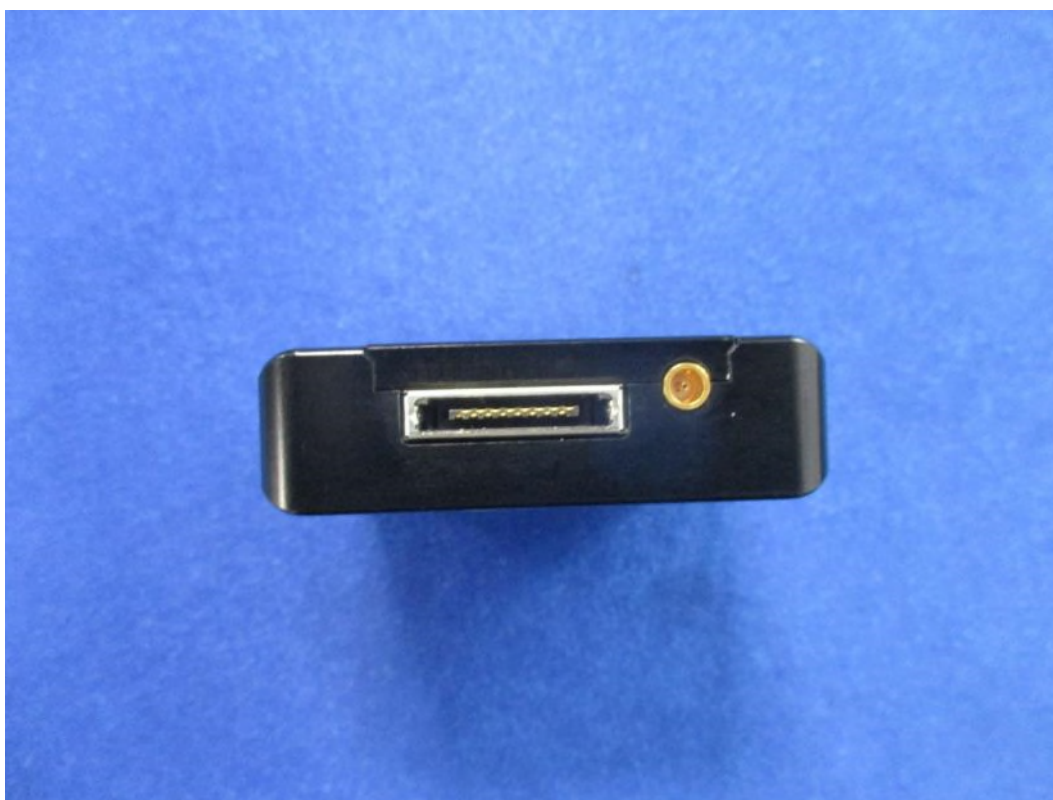
Photograph shows the EUT's power / control port and the SDI port
